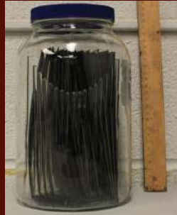
Leachate exposure: Both sides
